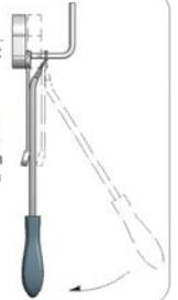
**2. Remove the (3) rubber plugs from each frame rail and enlarge the forward most hole to accept the supplied spacers and bolt heads.**
