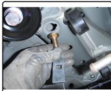
4. Raise hitch into position with exhaust and loosely install (5) supplied flange nuts.
