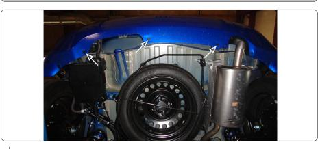
Mark and trim rear fascia. <u>Note</u>: Dimensions are approximate, confirm fit prior to trimming. See Fascia Trim Diagram
