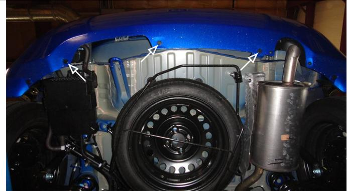
2. Mark and trim rear fascia. **Note:** Dimensions are approximate, confirm fit prior to trimming. See Fascia Trim Diagram
