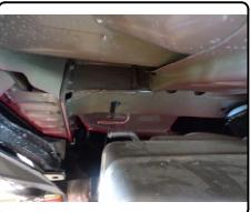
6. Raise hitch into position, feeding the fishwires through the hitch mounting holes.
