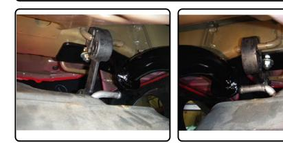
8. Install mounting straps using 1/2" carriage bolts and 1/2" flange nuts, as shown. Adjust hitch so the MOUNTING STRAPS are flush with the BUMPER BEAM.
