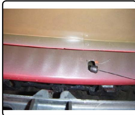
13. Re-install mounting straps into position, pulling fishwires through mounting strap holes. Loosely install the 1/2" carriage bolts and 1/2" flange nuts that attach mounting straps to hitch.
