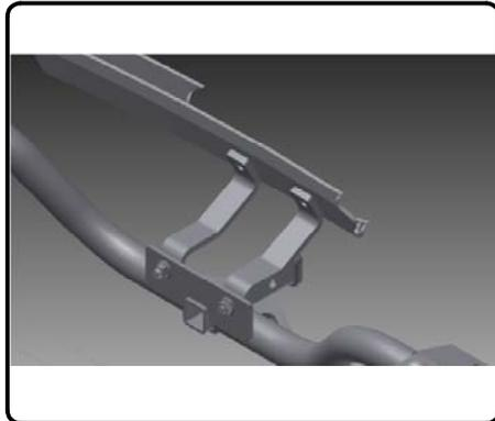
9. Tighten hardware installed in Step 8 using a 3/4" socket.
