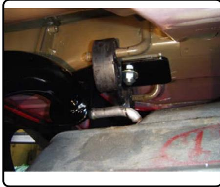
8. Install mounting straps using 1/2" carriage bolts and 1/2" flange nuts, as shown. Adjust hitch so the MOUNTING STRAPS are flush with the BUMPER BEAM.
