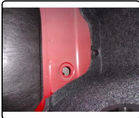
5. Using 20" fishwires, pull a CM-SP19 spacer and 1/2" carriage bolt through the TRUNK ACCESS HOLE on both sides. (See FISHWIRE TECHNIQUE diagram) Leave fishwires attached to bolts to prevent the hardware from being pushed back up into the frame.
