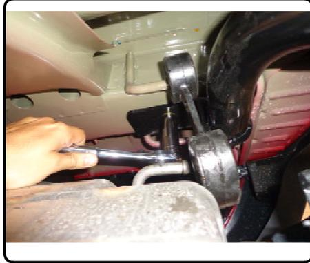
16. Raise exhaust back into position and re-install (6) rubber isolators removed in Steps 1&2.
