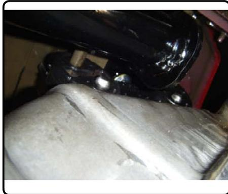
17. Reinstall (4) screws removed in Step 3 using a T20 Torx socket.
