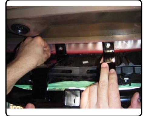
14. Remove fishwires from bolts installed in Step 12 and attach 1/2" flange nuts.
