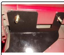
4. Torque 7/16" hardware to 59-ft lbs. Raise exhaust back into position
