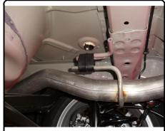
2. If a heat shield is present, you need to trim it to access the access hole in the frame.
