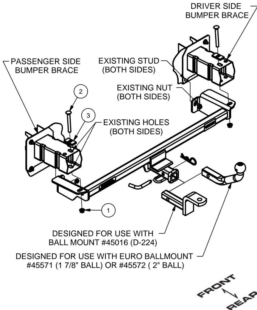
1. Remove existing 8mm nut from the inner most weld stud on frame flange, both sides.
