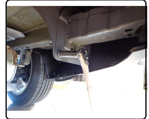
2. Raise hitch into position and secure the hitch front hole to the weld stud with nut removed in Step (1).
