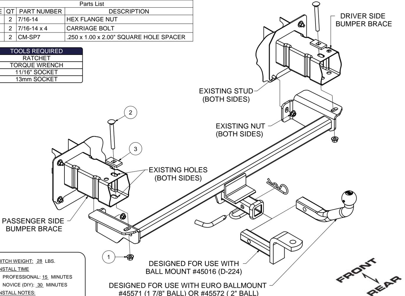
HITCH WEIGHT: 28 LBS.**INSTALL TIME**PROFESSIONAL: 15 MINUTESNOVICE (DIY): 30 MINUTES**INSTALL NOTES:****- NO DRILLING REQUIRED****INSTALLATION STEPS**
