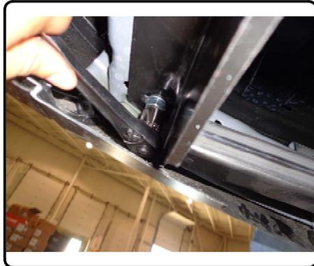
5. Torque all 7/16" hardware to 70 ft-lbs. Torque all 8mm hardware to 23 ft-lbs.
