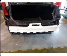
7. Remove bumper beam by removing (8) M8 bolts.
