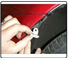
3. Remove small plastic panel between tail light and trunk opening. Remove exposed screw.
