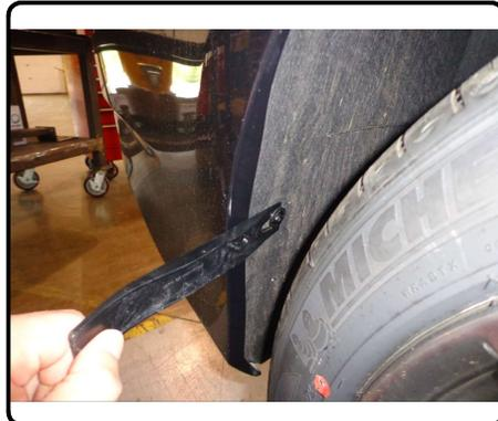
2. Remove (1) screw hidden behind the wheel well at the top of the fascia. Remove the plastic clip by prying it out with a flat head screw driver.
