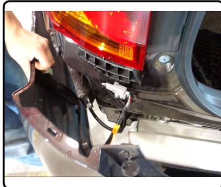
7. Remove bumper beam by removing (8) M8 bolts.
