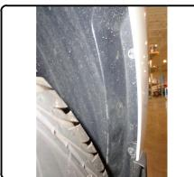
Disconnect fascia clips from under taillights to remove fascia. Gently pull fascia away from vehicle, making sure to carefully disconnect electrical connectors during removal. Set aside parts for reassembly.
