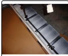
4. Drill out outboard passenger side rivet with 13/64" bit and trim 2 1/2" x 6" plastic area with shears or a rotary tool as shown. This will allow passenger side plate to sit flush when mounted.
