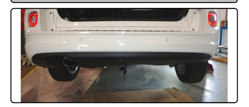
8. Trim approximatly 5" x 2 1/2" area at the center of the fascia as shown in the trim diagram. Reassemble the rear fascia by following Steps 1-2 in reverse.(2 bottom fascia mounting locations will now have been removed due to trim areas)
