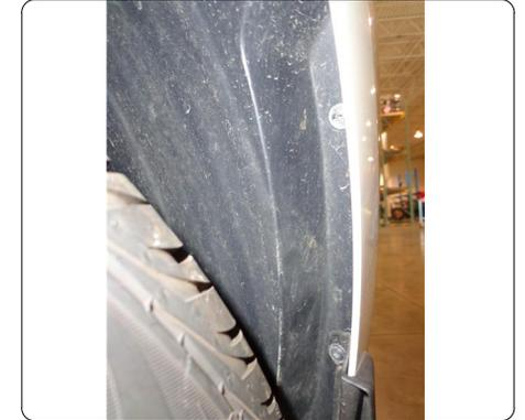
2. Disconnect fascia clips from under taillights to remove fascia. Gently pull fascia away from vehicle, making sure to carefully disconnect electrical connectors during removal. Set aside parts for reassembly.
