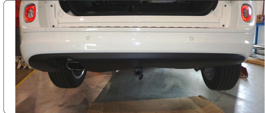
8. Trim approximately 5" x 2 1/2" area at the center of the fascia as shown in the trim diagram. Reassemble the rear fascia by following Steps 1-2 in reverse.
