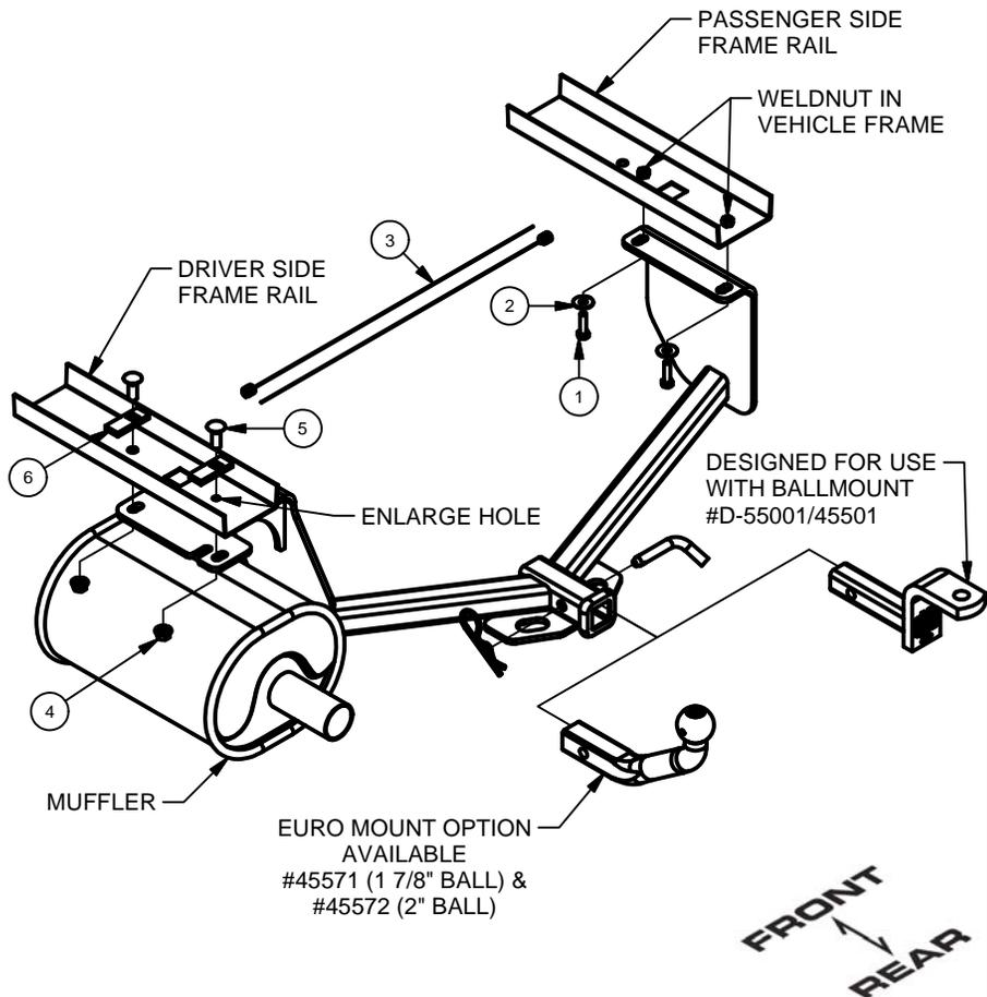
1. Lower exhaust by removing rubber exhaust hanger from hanger rod, two (2) places. Remove heat shield by removing four (4) hex nuts.
