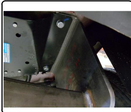
5. Trim heat shield as shown and install heat shield using two (2) hex nuts removed in step 1 and discard the other two (2) hex nuts. Raise exhaust back into position by reattaching rubber exhaust hangers to hanger rods.
