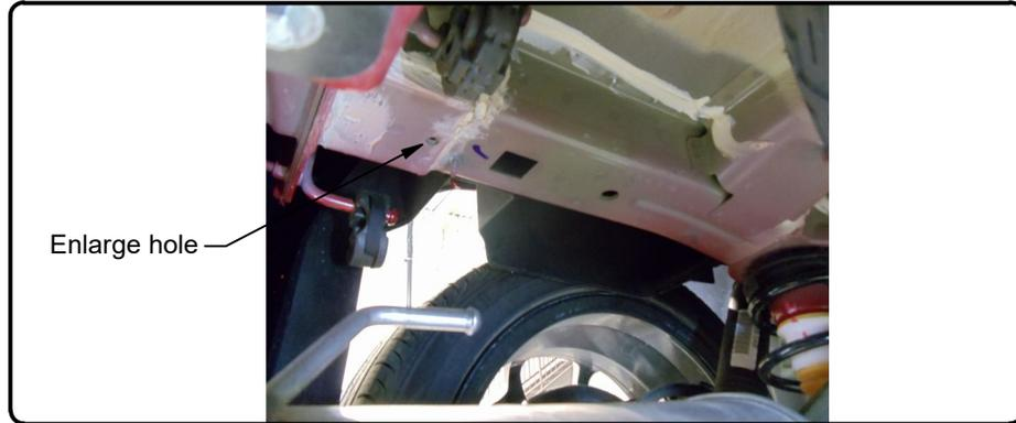
4. Raise hitch into position, taking care not to push carriage bolts back into frame and sandwiching hitch passenger side plate between frame rail and spare tire control box, if equipped. Install M8 hex bolts and 7/16" conical toothed washers into weldnuts in passenger side frame rail. Install flanged hex nuts onto carriage bolts in driver side frame rail. Torque all 7/16" fasteners to 59 lb.-ft.; Torque all M8 fasteners to 23 lb.-ft.
