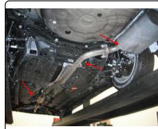
6. Remove the (2) tie down / exhaust hanger brackets from the frame using a 14mm socket. Return brackets to vehicle owner but keep hardware and rubber isolators for step 9.
