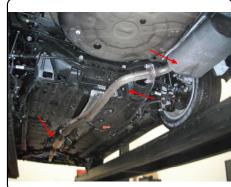
13. ON SINGLE EXHAUST MODEL ONLY: Trim the underbody panel as shown in the diagrams below for the hitch to pass through.
