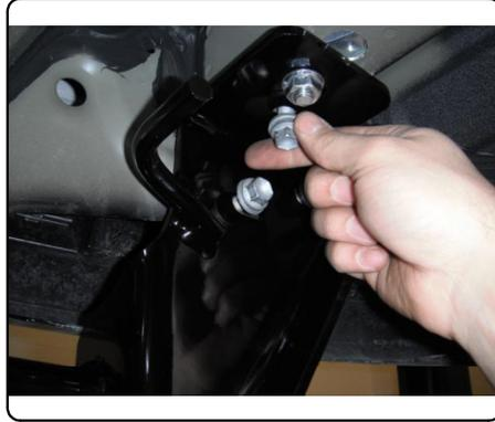
11. Torque all 10mm fasteners to 56 lb-ft and all 7/16" fasteners to 70 lb-ft.
