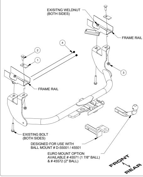
1. Remove existing bolt from driver and passenger side of vehicle. Retain bolt for hitch installation.
