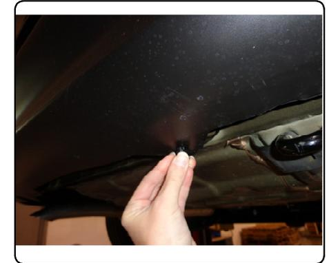
2. Use a die grinder to enlarge the rear hole in the driver side framerail. This will be used for the access hole for fishwiring mounting hardware.
