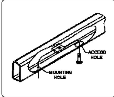
4. Reverse fishwire rearward 1/2" mounting hardware into the frame access hole as shown.
