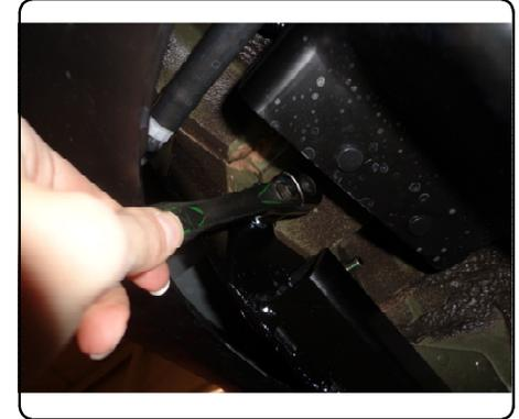
6. Using 1/2" carriage bolt, nut and spacer, attach rear hitch plate to vehicle tow loop.
