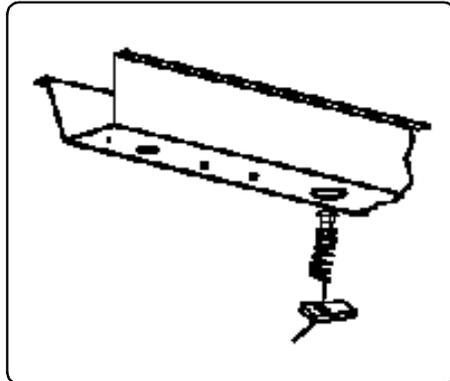
5. Raise hitch into position, attaching to the fishwired hardware on the driver side. 3/8" hardware will push through the rear of the vehicle frame on the passenger side and attach with a 9/16" socket as shown. Hold tightly on the back side with a boxed end wrench to secure.
