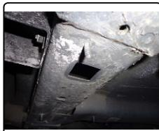
4. Using a 7/16" drill bit, enlarge hole rearward of square holes on driver side frame rail. Fishwire 7/16" carriage bolts and spacer blocks up through square hole and down through mounting holes as shown.
