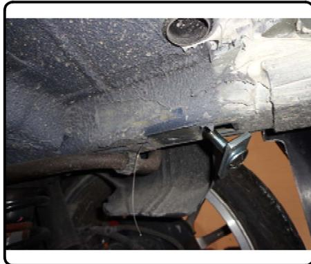
5. Raise hitch into position and secure hardware, taking care not to push the carriage bolts back up into frame rails.
