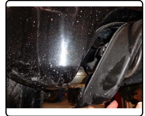
2. Lower exhaust by removing rubber exhaust hangers from hanger rods in (1) location on the driver side and (1) location on the passenger side. The additional exhaust hanger bracket on the passenger side will need to be completely removed from the vehicle frame (if equipped). Remove and return the bracket and hardware to the owner.
