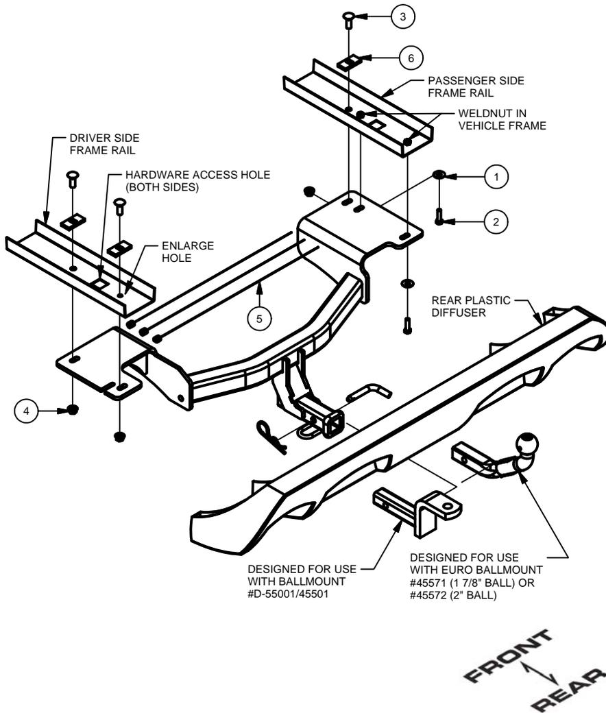
1. Remove rear plastic diffuser by removing (2) T15 torx and (2) 5/16 screws from the bottom and by carefully disconnecting clips from inside of plastic. Pull piece gently away from rear of vehicle to remove. Set aside for trimming and reassembly.
