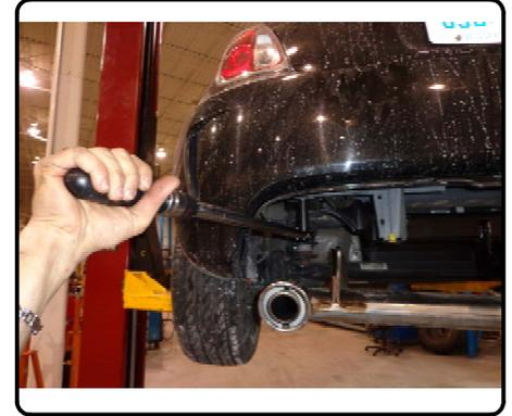
6. Raise exhaust back into position and secure to vehicle hangers.
