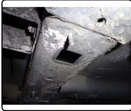
4. Using a 7/16" drill bit, enlarge hole rearward of square holes on driver side frame rail. Fishwire 7/16" carriage bolts and spacer blocks up through square hole and down through mounting holes as shown.
