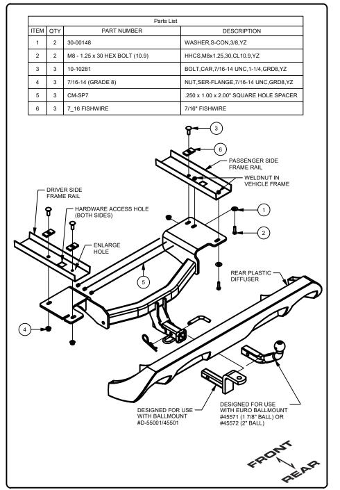
1. Remove rear plastic diffuser by removing (2) T15 torx and (2) 5/16 screws from the bottom and by carefully disconnecting clips from inside of plastic. Pull piece gently away from rear of vehicle to remove. Set aside for trimming and reassembly.
