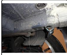
5. Raise hitch into position and secure hardware, taking care not to push the carriage bolts back up into frame rails.
