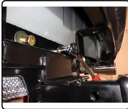
5. Mark and trim both heat shield and plastic rear fascia as shown. Bend heat shield up into its concealed position. Reattach plastic fascia by clipping back onto vehicle and securing both screws on sides of vehicle.
