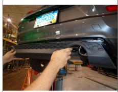
2. Fishwire (2) 1/2"carriage bolts and spacer blocks through driver side access hole in bumper beam.
