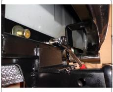
5. Mark and trim both heat shield and plastic rear fascia as shown. Bend heat sheild up into its concealed position. Reattach plastic fascia by clipping back onto vehicle and securing both screws on sides of vehicle.
