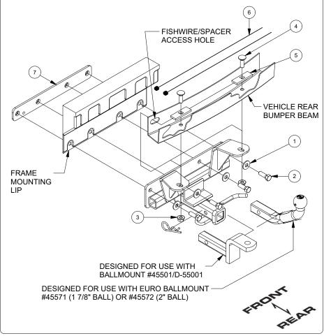
1. Remove plastic fascia from rear of vehicle to gain access to hitch mounting locations. First, remove (2) screws from plastic mounting brackets using a T-25 Torxbit socket. Then, un-clip plastic from vehicle and gently pull back to remove.
