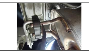
2. Enlarge hole at the end of each frame rail to accommodate square hole spacers and 7/16" carriage bolts.
