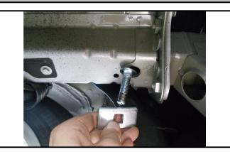
4. Raise hitch into position and loosely attach 7/16" hex flange nuts to carriage bolts.
