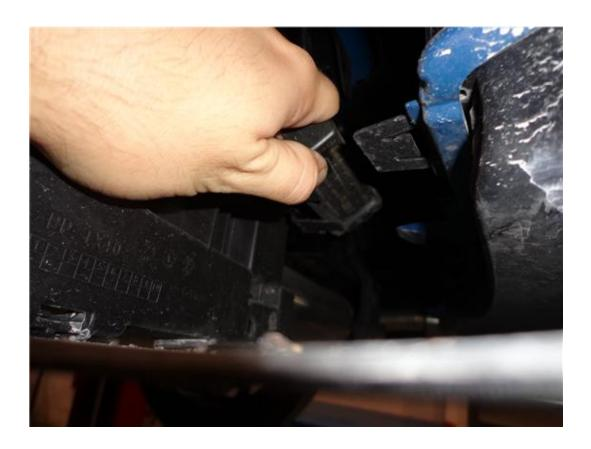
2. Remove (1) plastic rivet each side of the underside of the bumper cover by using a pair of side cutters and cutting off the top of the rivet. Discard removed rivets.
