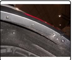
6. Lightly pull the plastic fender flare back on each side exposing an 8mm bolt and the reflector light wiring. Unbolt the 8mm bolt with a wrench and disconnect the reflector light and let hang.
