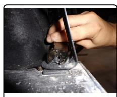
4. Remove (2) 7mm bolts from each side of the wheel well that secure the bumper fascia.
