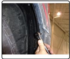
5. Remove the first (2) plastic rivets above the 7mm bolts previously removed, by pushing the center of the rivet through with a small punch and prying the head of the rivet out with a flat head screw driver.
