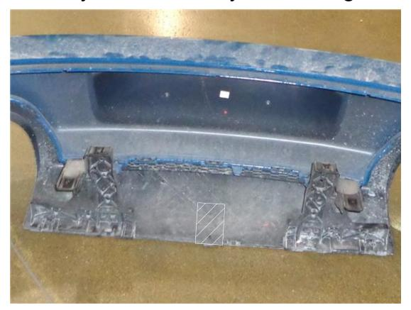
12. Reinstall the bumper cover by following the disassembly steps 1-10 in reverse. Replace (6) removed plastic rivets with those supplied in the hardware kit attach using a plasticrivet gun.
