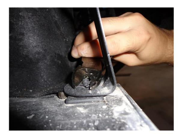
3. Remove (2) 7mm bolts from each side of the wheel well that secure the bumper fascia.
