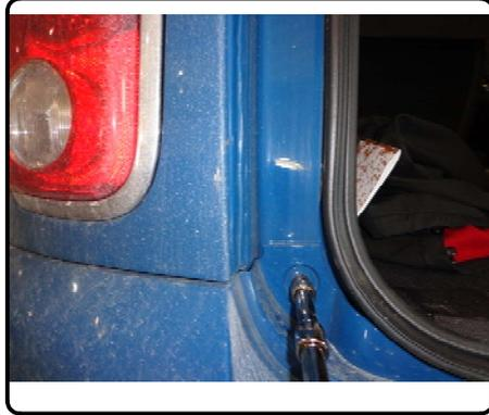
8. Remove (4) 10mm plastic nuts from the bumper braces on the underside of the vehicle as shown.
