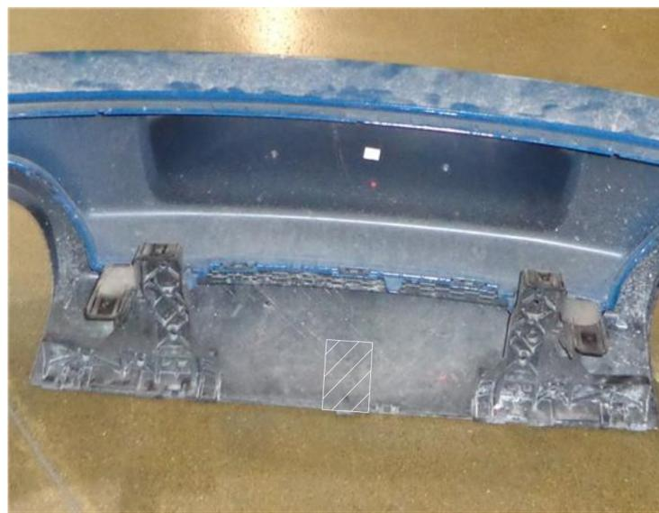
12. Reinstall the bumper cover by following the disassembly steps 1-10 in reverse. Replace (6) removed plastic rivets with those supplied in the hardware kit attach using a plasticrivet gun.
