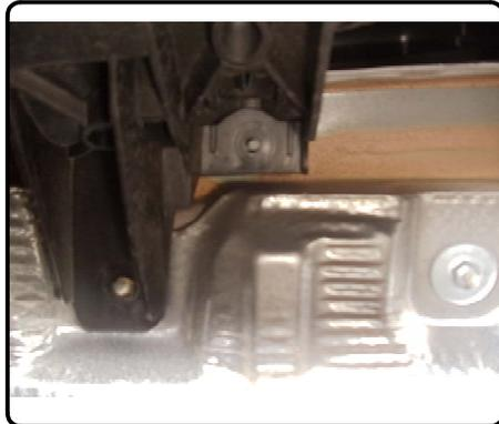
9. To remove bumper cover, gently pull each side of the bumper fascia rearward of the vehicle and set bumper cover aside. (Models with reverse sensors will need to disconnect (4) connectors)
