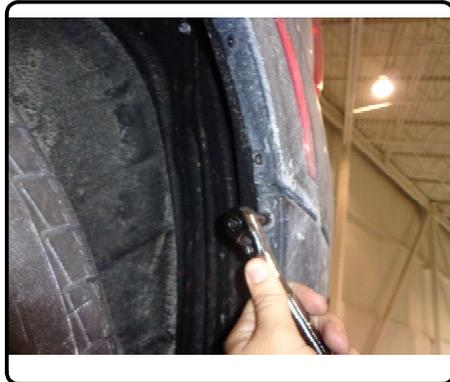
5. Remove the first (2) plastic rivets above the 7mm bolts previously removed, by pushing the center of the rivet through with a small punch and prying the head of the rivet out with a flat head screw driver.
