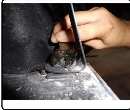
4. Remove (2) 7mm bolts from each side of the wheel well that secure the bumper fascia.
