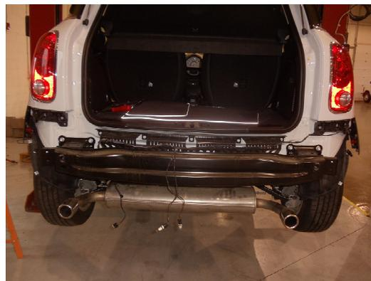
9. Remove the (6) 15mm flange nuts attaching the bumper to the vehicle, remove bumper and set aside.
