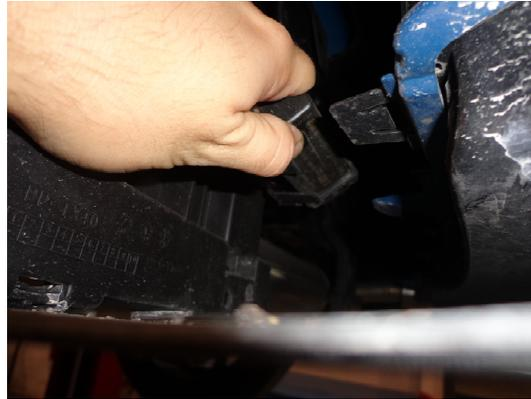
2. Remove (1) plastic rivet each side of the underside of the bumper cover by using a pair of side cutters and cutting off the top of the rivet. Discard removed rivets.
