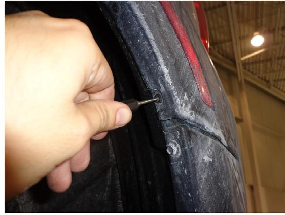
5. Lightly pull the plastic fender flare back on each side exposing an 8mm bolt and the reflector light wiring. Unbolt the 8mm bolt with a wrench and disconnect the reflector light and let hang.
