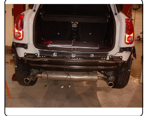
10. Remove the (6) 15mm flange nuts attaching the bumper to the vehicle, remove bumper and set aside.
