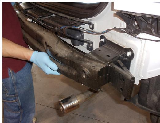
**PERIODICALLY CHECK THIS RECEIVER HITCH TO ENSURE THAT ALL FASTENERS ARE TIGHT AND THAT ALL STRUCTURAL COMPONENTS ARE SOUND.**
