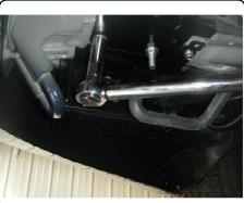
6. Reinstall exhaust isolator hangers. Install is now complete.
