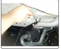
INSERT COILED END OF FISHWIRE TOOL THROUGH HITCH MOUNTING HOLE IN VEHICLE FRAME RAI END OF FISHWIRE THROUGH SPACER AND HREAD BOLT INTO COLL KINK WIRE TO KEEP SPACER SEPERATE FROM BOLT AS SHOWN, PULL CCES SOLT THROUGH FRAME ND OUT MOUNTING HOL JSE FISHWIRE TO GUIDE ITCH DURING MOUNTING AND PREVENT LOSS OF BOLT / PACER INSIDE FRAME RAIL \*NOTE: SOME VEHICLES MAY FISHWIRE THROUGH END OF FRAME\*
