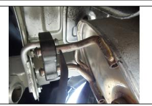
2. Enlarge hole at the end of each frame rail to accommodate square hole spacers and 7/16" carriage bolts.
