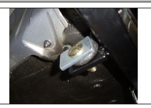
6. Torque 7/16" hardware to 70 lb-ft. Torque 1/2" hardware to 110 lb-ft.
