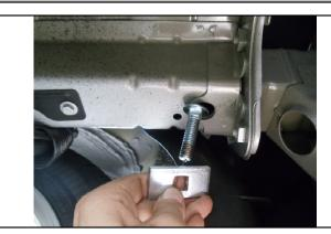
4. Raise hitch into position and loosely attach 7/16" hex flange nuts to carriage bolts.
