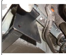
5. Install 1/2" carriage bolt with large square hole spacer through tow hook and support bar on hitch and fasten with 1/2" flange nut, as shown.
