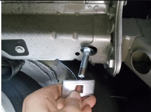
5. Install 1/2" carriage bolt with large square hole spacer through tow hook and support bar on hitch and fasten with 1/2" flange nut, as shown.
