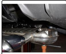
4. Remove heat shield by removing (8) nuts which secure it to the vehicle. Retain (6) nuts for reinstallation after heat shield trimming.
