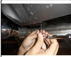
2. Lower exhaust by first removing (2) bolts on each side from the end of the vehicle frame rails that secure the exhaust hanger brackets. Remove brackets from hanger pegs on muffler. Then remove the rubber exhaust hangers, (4) places forward of mufflers (3) places on Coupe models.
