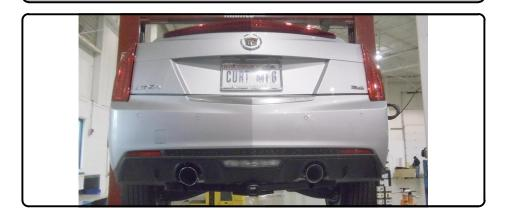
9. Raise hitch and exhaust into position simultaneously, being careful not to push bolts back into frame. Secure with 1/2" flange hex nuts. Torque all 1/2" hardware to 110 lb-ft. Follow Step 1 in reverse order to raise hitch back into position. Reattach exhaust support strap if removed in Step 3.
