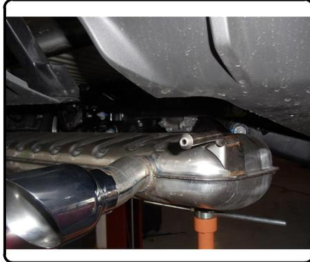
4. Remove heat shield by removing (8) nuts which secure it to the vehicle. Retain (6) nuts for reinstallation after heat shield trimming.
