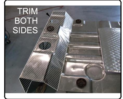
7. Trim vehicle fascia as shown on each side of the vehicle to allow for hitch side plate reinstallation, approximately 1-3/8" each side.
