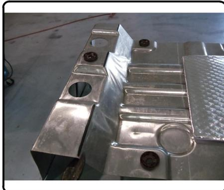
5. Cut off stud from each frame rail that secured the heat shield.
