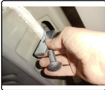
9. Raise hitch and exhaust into position simultaneously, being careful not to push bolts back into frame. Secure with 1/2" flange hex nuts. Torque all 1/2" hardware to 110 lb-ft. Follow Step 1 in reverse order to raise hitch back into position. Reattach exhaust support strap if removed in Step 3.
