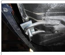
9. Raise hitch into position by raising passenger side of hitch over exhaust first. (The heat shield will be sandwich between the side plate and frame rail.) Loosely install 1/2-13 flanged nut onto carriage bolt from step 7.
