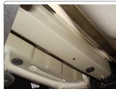
4. Locate and remove rear rubber cap from driver and passenger side frame rail. (Discard cap on Sedan vehicles only.)
