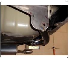
10. Loosely install 1/2-13 flanged nut onto carriage bolt from both frame rails.
