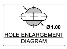
6. Reverse fishwire 1/2-13 carriage bolts and CM-SP6 spacers through the enlarged access hole, both sides.
