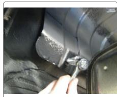
8. Install 1/2-13 carriage bolt and CM-SP4 spacer through top of existing vehicle tow loop, as shown.
