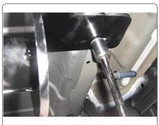
12. On Coupe models, trim plastic on drivers side of vehicle as shown and reinstall back into position.
