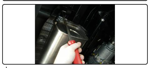
2. Enlarge existing hole under frame rail to 1" as shown.
