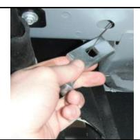
4. Place remaining 2" carriage bolt through hitch onto tow loop and place small CM-SP12 spacer on bottom of tow loop. Raise passenger side and secure with flange nut.
