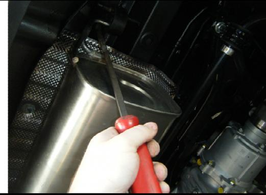
2. Enlarge existing hole under frame rail to 1" as shown.
