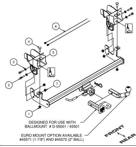
1. Enlarge existing hole to allow 7/16" carriage bolts and SP7 spacers to pass through, both sides.
