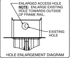
2. Reverse fishwire 7/16" carriage bolts and SP7 spacers through enlarged access holes, both sides.
