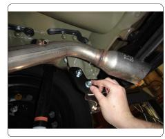
5. Torque all 7/16" hardware to 70 ft-lbs. Torque all 3/8" hardware to 45 ft-lbs.
