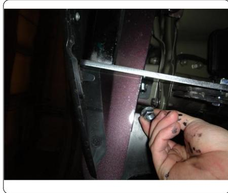
4. Align holes in side plates with holes in tow loops and secure using 3/8" hex bolts, 3/8" washers and 3/8" hex flange nuts, as shown.
