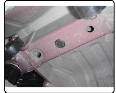
2) Fishwire 7/16" carriage bolts and spacers into position first and reverse fishwire the 1/2" carriage bolts and spacers into position afterward. (enlarge access hole as necessary)
