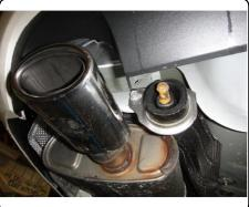
2. If a heat shield is present you need to trim it to access the access hole in the frame. <u>Note</u>: Dimensions are approximate, confirm prior to trimming.
