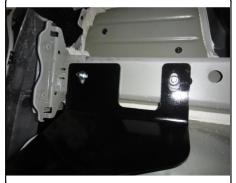
4. Torque 7/16" hardware to 70 ft-lbs. Raise exhaust back into position.
