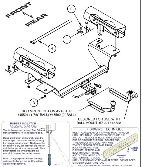
Lower exhaust by removing (2) rubber isolators from the muffler towards the center of the vehicle and by removing the bolt securing the rearmost hanger to the frame.
