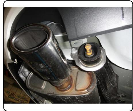
2. If a heat shield is present you need to trim it to access the access hole in the frame. **Note:** Dimensions are approximate, confirm prior to trimming.
