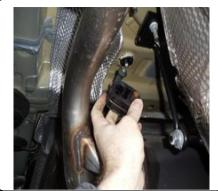
2. Lower the exhaust by removing the muffler bracket as shown and allow to hang while still supporting it.
