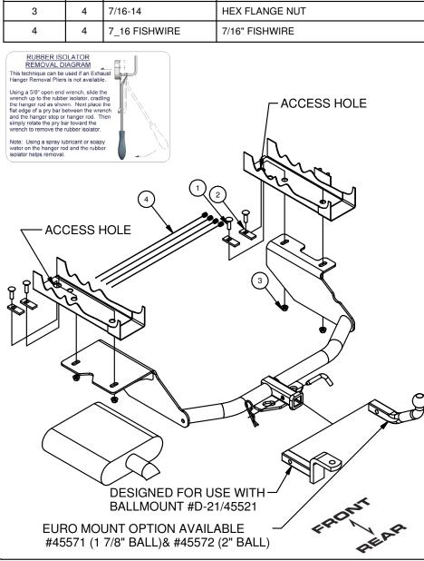
1. Support the exhaust system to avoid damage during installation. Remove the rubber isolators located behind the spare tire cage on both drivers side and passenger side. (See Rubber isolator removal diagram.)
