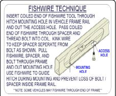
6. Taking care not to push the fishwired hardware into the frame rails, raise the hitch into position, aligning the fishwired hardware with the slots in the hitch side plates. Loosely secure the hitch to the vehicle using the (4) 7/16" hex flange nuts as shown.
