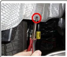
4. Using Aviation shears, trim the heat shield as shown and reinstall the unhatched section on the trunk pan. (See heat shield trimming)
