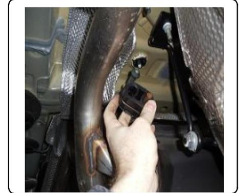
2. Lower the exhaust by removing the muffler bracket as shown and allow to hang while still supporting it.
