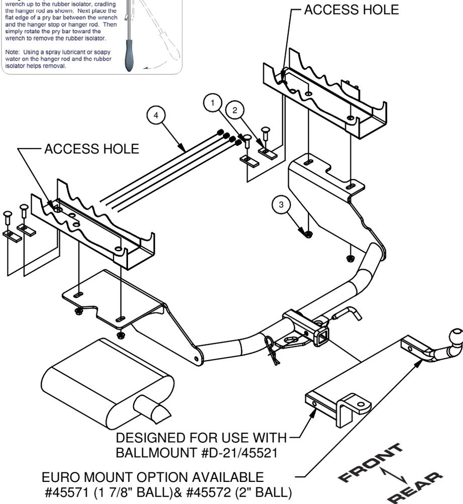
1. Support the exhaust system to avoid damage during installation. Remove the rubber isolators located behind the spare tire cage on both drivers side and passenger side . (See Rubber isolator removal diagram.)
