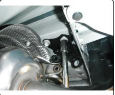
2. Remove existing bolts from tow loop. Return tow loop and bolts to owner. **NOTE:** Access bolts through tow loop cut out in the underbody panel on standard Prius models.
