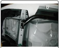
4. Clamp the passenger side plate between the frame rail and exhaust bracket. Secure using M12 - 1.25 X 40mm bolts with 1/2" conical toothed washers, as shown above.
