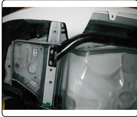
4. Clamp the passenger side plate between the frame rail and exhaust bracket. Secure using M12 - 1.25 X 40mm bolts with 1/2" conical toothed washers, as shown above.
