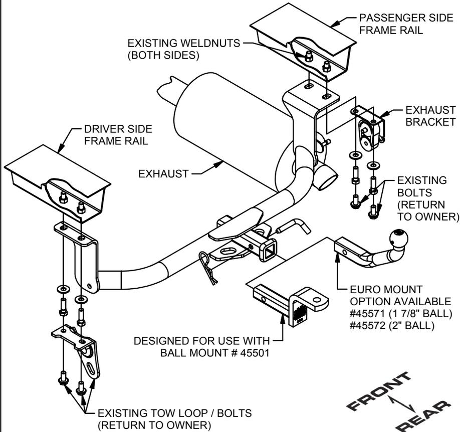
1. Remove existing bolts from rearmost exhaust hanger to lower exhaust. Return bolts to owner. **NOTE:** For ease of installation rearmost remove rubber isolator. See RUBBER ISOLATOR REMOVAL DIAGRAM.
