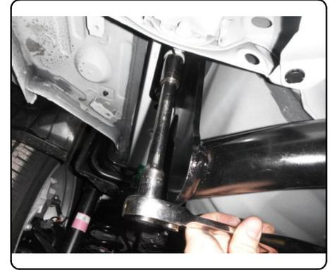
6. Reinstall rubber isolator (if it was removed in step 1).
