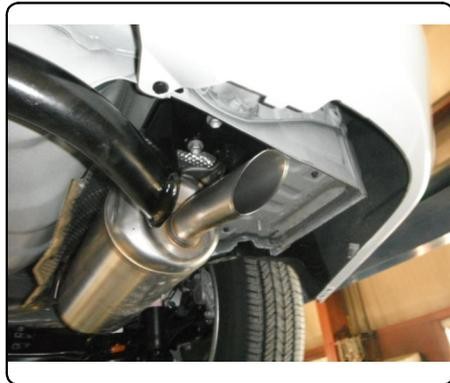
5. Torque all 12mm fasteners to 86 ft-lbs.
