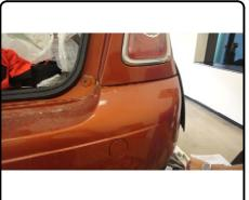
14. With bumper back to installed position, mark out the bumper for trimming to access the receiver hitch as shown in the diagram below. NOTE: These dimensions are for referance only and should be verified on the vehicle. Drilling a small hole will help verify location.
