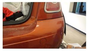
14. With bumper back to installed position, mark out the bumper for trimming to access the receiver hitch as shown in the diagram below. NOTE: These dimensions are for referance only and should be verified on the vehicle. Drilling a small hole will help verify location.
