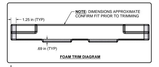
10. After trimming foam block insert into the bumper beam and confirm fit. Raise the hitch into position by aligning holes with weldnuts. **Note:** Heat shield may need to be formed around hitch. Spare tire may need to be loosened and plastic tire cradle adjusted to accommodate tow loops.
