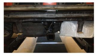
11. Sandwich the hitch between the bumper beam and the rear of the car. Secure hitch using (8) existing M8 bolts removed in Step 6 and 3/8" conical toothed washers. Torque all M8 hardware to 23 ft-lbs.
