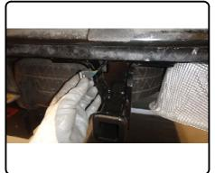
13. Align bumper cover and pull back on the fender flairs. Re-attach side marker bulbs to fender flairs. Reconnect rear sensors. Reinstall all (11) fasteners removed previously and snap fender flairs back into place.
