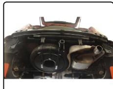
12. Your car is ready for re-assembly. Reconnect the wiring harness to the bumper beam by reinstalling the push fasteners removed in Step 7. In reconnecting the backup/center tail light, pass the wire over the top of the hitch and run the connector through the hole in the hitch as shown. **Note:** Keep wiring harness clear of the exhaust and heat shield.
