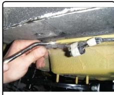
8. Remove the (8) M8 bolts and lower bumper beam assembly from vehicle. If present, remove divider panel from bumper beam and return to owner.
