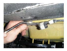
8. Remove the (8) M8 bolts and lower bumper beam assembly from vehicle. If present, remove divider panel from bumper beam and return to owner.
