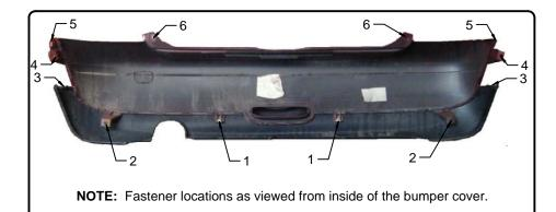
2. Using a phillips screwdriver remove (4) fasteners securing the mudflap, two each side of vehicle. Using a flat blade screwdriver remove the (4) clips from the mudflap, two each side. **NOTE:** If needed you may remove rear wheels to access fasteners.
