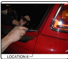
6. If your vehicle is equipped with a rear light or rear sensors, disconnect the wiring harness from the back of the bumper cover and remove the light from the back side by depressing tabs on both sides of the light. Pull back and up on the center of the cover to release it from the mounting tab. Place bumper cover in a safe place to prevent damage.
