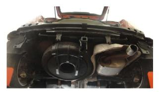
12. Your car is ready for re-assembly. Reconnect the wiring harness to the bumper beam by reinstalling the push fasteners removed in Step 7. In reconnecting the backup/center tail light, pass the wire over the top of the hitch and run the connector through the hole in the hitch as shown. **Note:** Keep wiring harness clear of the exhaust and heat shield.
