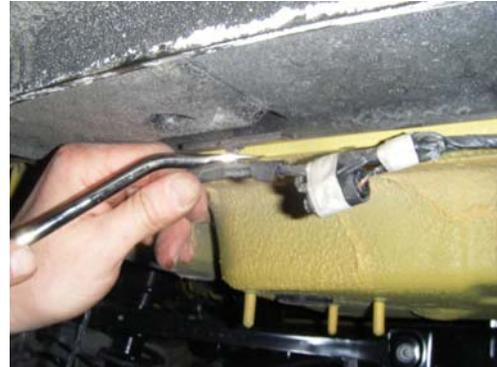
8. Remove the (8) M8 bolts and lower bumper beam assembly from vehicle. If present, remove divider panel from bumper beam and return to owner.
