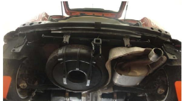
12. Your car is ready for re-assembly. Reconnect the wiring harness to the bumper beam by reinstalling the push fasteners removed in Step 7. In reconnecting the backup/center tail light, pass the wire over the top of the hitch and run the connector through the hole in the hitch as shown. **Note:** Keep wiring harness clear of the exhaust and heat shield.
