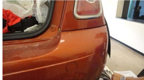
14. With bumper back to installed position, mark out the bumper for trimming to access the receiver hitch as shown in the diagram below. NOTE: These dimensions are for reference only and should be verified on the vehicle. Drilling a small hole will help verify location.
