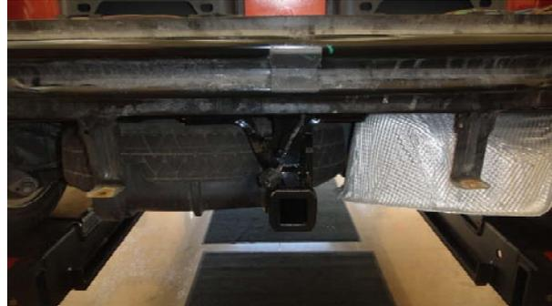
11. Sandwich the hitch between the bumper beam and the rear of the car. Secure hitch using (8) existing M8 bolts removed in Step 6 and 3/8" conical toothed washers. Torque all M8 hardware to 23 ft-lbs.
