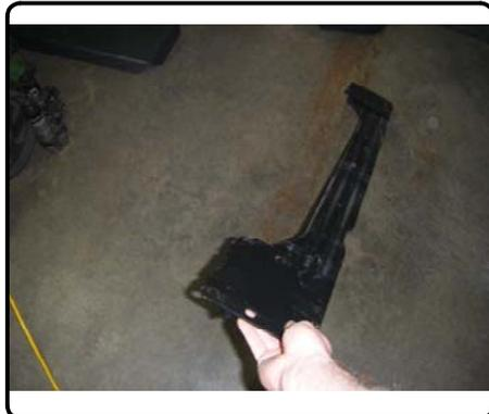
9. If present, remove hard foam energy absorber and trim to allow proper fit. (See trim diagram) **Note:** Some models may have soft foam and not require trimming.
