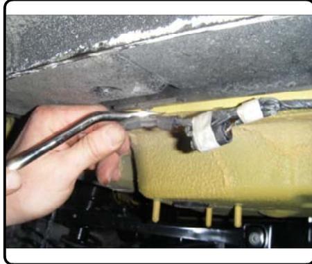
8. Remove the (8) M8 bolts and lower bumper beam assembly from vehicle. If present, remove divider panel from bumper beam and return to owner.
