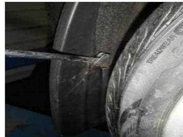
3. Inside wheel well remove (2) hex head fastener from location 4, one each side. Pull back the wheel well liner to access the (2) push fasteners that hold the rear wheel arch to the rear bumper cover from location 3, one each side. Remove fasteners by pushing the inner piece down to expose the head. Use a screw driver to pry out of position.
