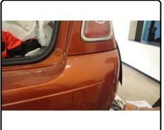
14. With bumper back to installed position, mark out the bumper for trimming to access the receiver hitch as shown in the diagram below. NOTE: These dimensions are for referance only and should be verified on the vehicle. Drilling a small hole will help verify location.
