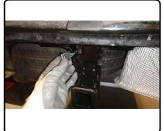
13. Align bumper cover and pull back on the fender flairs. Re-attach side marker bulbs to fender flairs. Reconnect rear sensors. Reinstall all (11) fasteners removed previously and snap fender flairs back into place.
