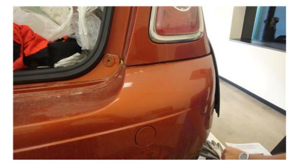
14. With bumper back to installed position, mark out the bumper for trimming to access the receiver hitch as shown in the diagram below. NOTE: These dimensions are for referance only and should be verified on the vehicle. Drilling a small hole will help verify location.
