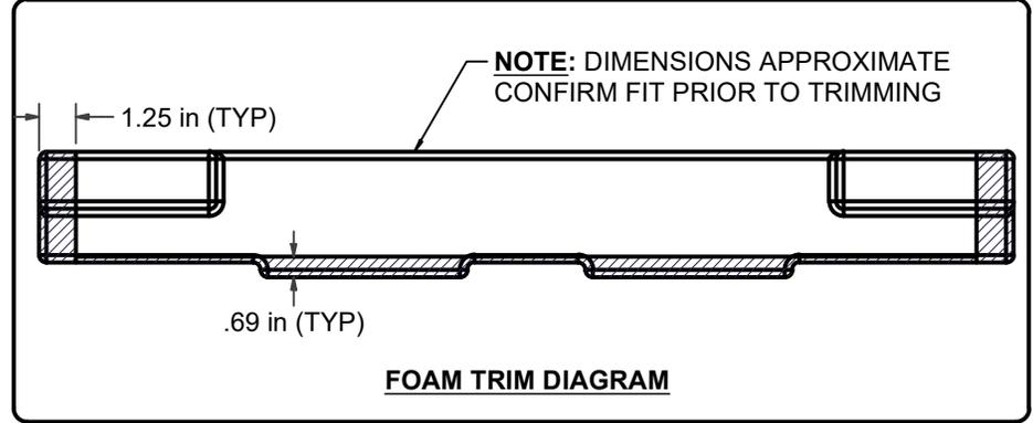
10. After trimming foam block insert into the bumper beam and confirm fit. Raise the hitch into position by aligning holes with weldnuts. **Note:** Heat shield may need to be formed around hitch. Spare tire may need to be loosened and plastic tire cradle adjusted to accommodate tow loops.
