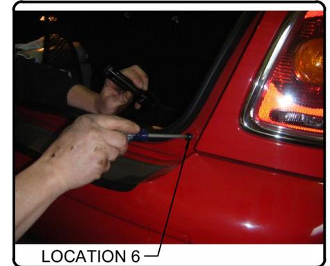
6. If your vehicle is equipped with a rear light or rear sensors, disconnect the wiring harness from the back of the bumper cover and remove the light from the back side by depressing tabs on both sides of the light. Pull back and up on the center of the cover to release it from the mounting tab. Place bumper cover in a safe place to prevent damage.
