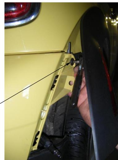
5. Using a 10mm socket remove (2) fasteners from under bumper cover from location 1. Remove the final (2) fasteners from location 6, these are visible when you open the rear hatch.
