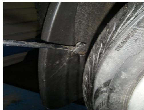
3. Inside wheel well remove (2) hex head fastener from location 4, one each side. Pull back the wheel well liner to access the (2) push fasteners that hold the rear wheel arch to the rear bumper cover from location 3, one each side. Remove fasteners by pushing the inner piece down to expose the head. Use a screw driver to pry out of position.
